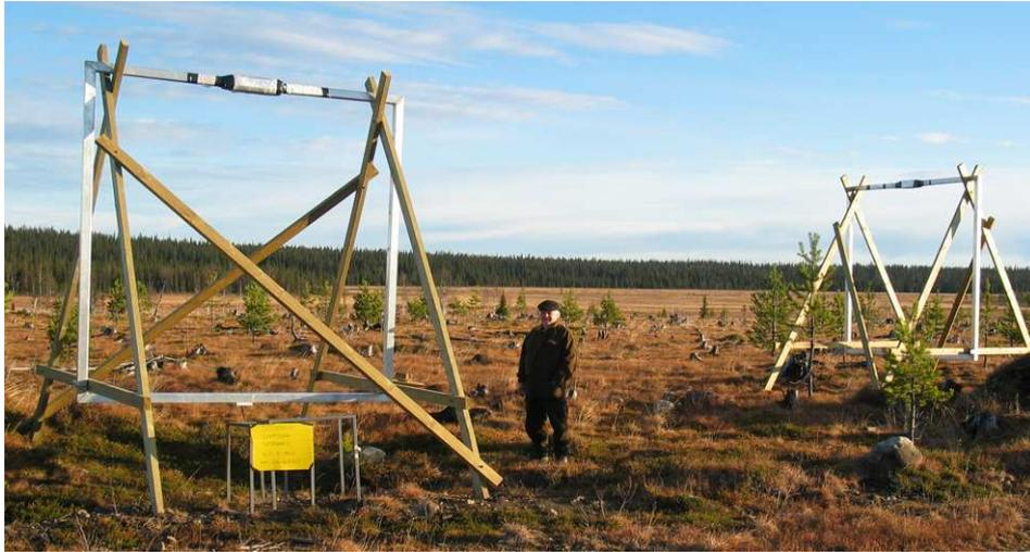
Figure 2.3: The UEV2300 ULF-ELF-VLF receiver antennas. The size of the loop is  $3 \times 3 \text{ m}^2$  with 2 times 128 turns, i.e. the effective area is  $2300 \text{ m}^2$ . The person in the photo is Prof. Tauno Turunen.
