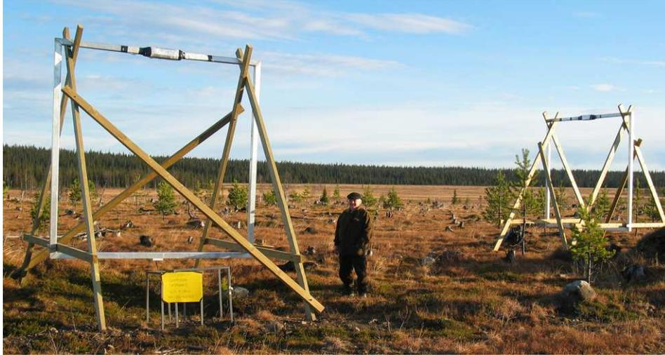
Figure 2.3: The UEV2300 ULF-ELF-VLF receiver antennas. The size of the loop is  $3 \times 3 \text{ m}^2$  with 2 times 128 turns, i.e. the effective area is  $2300 \text{ m}^2$ . The person in the photo is Prof. Tauno Turunen.
