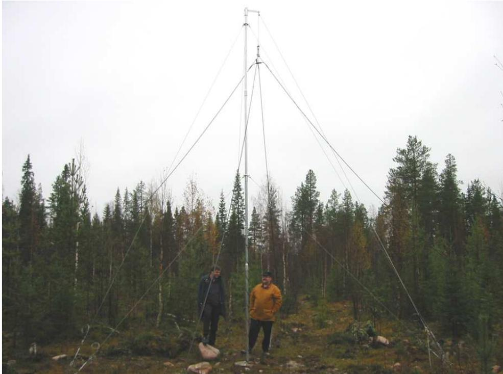
Figure 2.1: The ELF-VLF receiver antenna of IGY type. It has two orthogonal loops suspended from an aluminium mast. This antenna was located at Perunkajärvi, Rovaniemi until June 2005 and is at Pittiövaara, Sodankylä since September 2005, and belongs to BAS. The persons are Dr. Mark Clilverd (left) from BAS and the author of this thesis. (Photo by Thomas Ulich)
