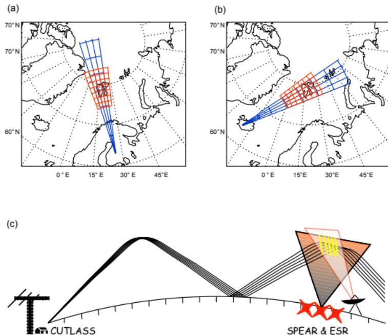
**Fig. 5.** Summary of CUTLASS experimental operations. (a) Scanning pattern for CUTLASS Finland, (b) scanning pattern for CUTLASS Iceland, (c) schematic of 1.5-hop propagation path between CUTLASS radar and SPEAR/ESR sites.
