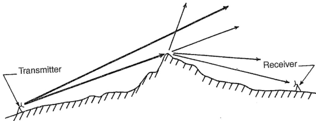
Figure: Terrain diffraction (Levis, 2010).
