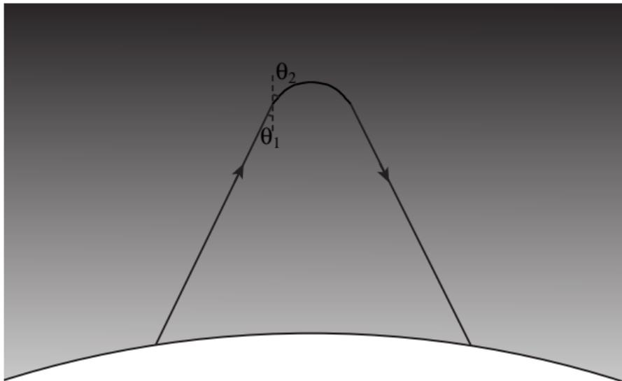
**Figure:** Oblique transmission (for a frequency that is not penetrating the ionosphere).
