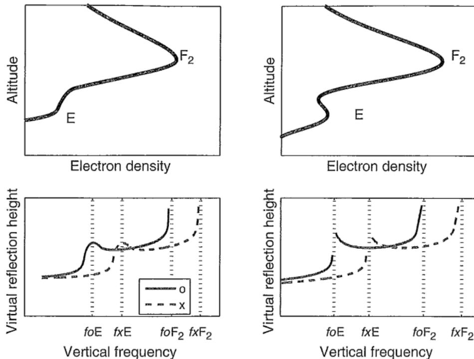
Figure: Electron density profiles and corresponding ionograms.
