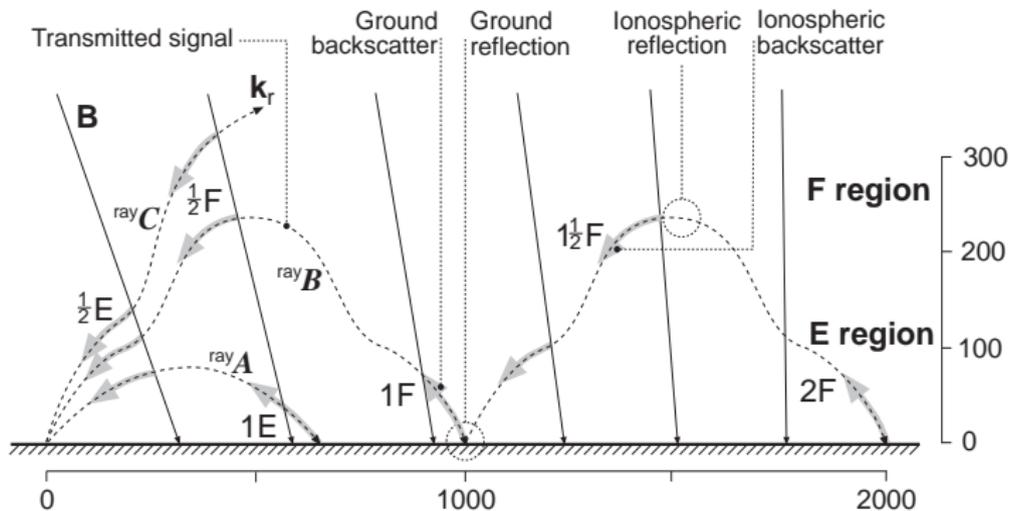
Figure: Different ray paths for the HF signal (Milan et al., 1997).
