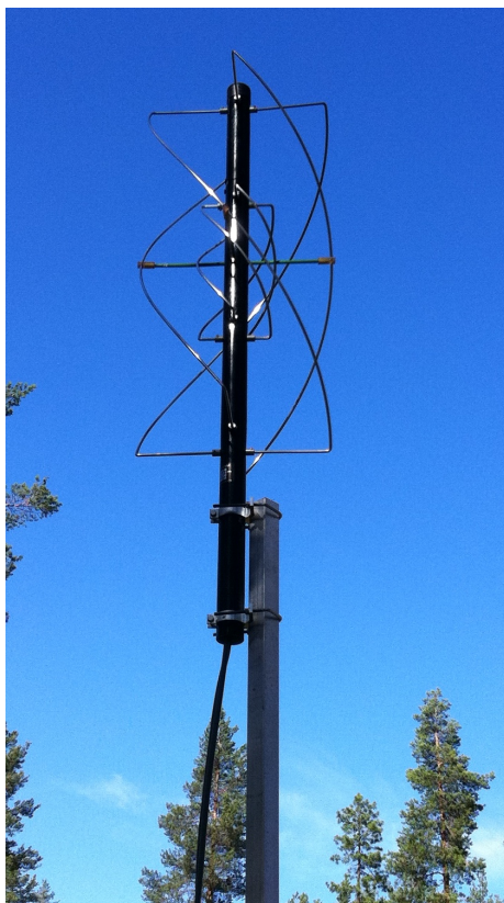
Figure 2: The dual band 150/400 MHz quadrifilar helical antenna.
