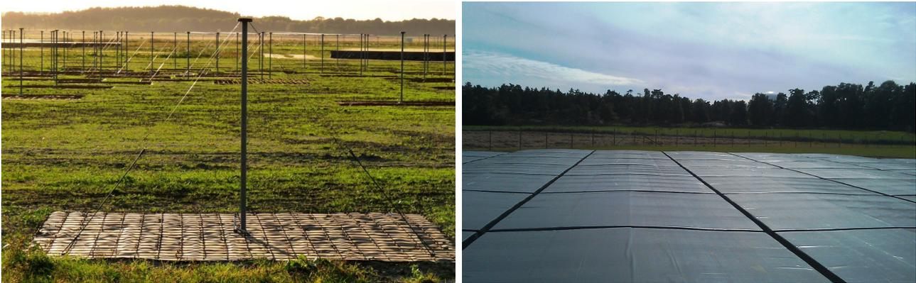
Figure 1: LBA elements (left) and HBA tiles (right) on field. ©Menno Norden
